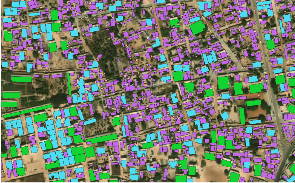
Figure 5: Colored polygons represent rooftops categorized by building size and associated energy demand. Green polygons indicate large buildings, teal represents medium buildings, and purple denotes small buildings. Very small structures, shown in light beige, are excluded from the energy demand estimation.
